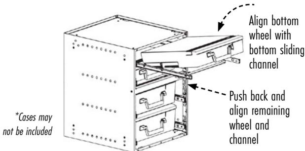
**D** If you have cases, carefully reinstall the RolaCases into the roller bearing slides by pushing gently without damaging the slides and the cases, refer to previous image
