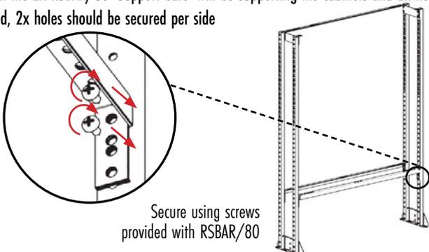
Secure using screws provided with RSBAR/80
