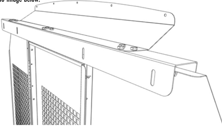
**B** Once the partition unit is fully assembled, use two people to lift the assembly into the van via the side door and position into place
