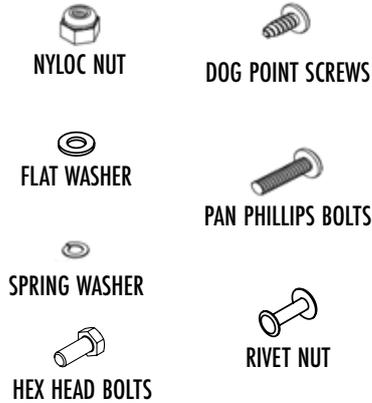
The RolaCase Partition Kit for the Ram ProMaster (Part#: **RSCGBRPM118136159**) is made up of the following 7 parts that need to be located and assembled together with the hardware provided:
