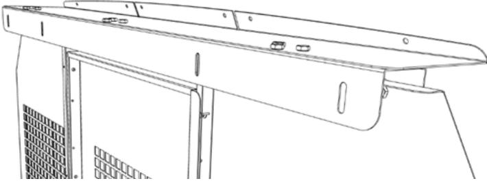
**B** Locate the Centre Panel, R/H side Panel, and the L/H side Panel. If you have purchased the "Swing Door & Lock Kit", please follow the instructions in that kit, otherwise assemble the three products together using 14x "M6 x 12mm" bolts and Nyloc nuts provided, refer to image below:
