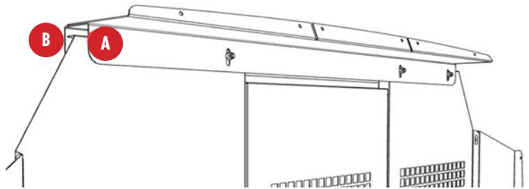
**D** Locate the R/H setback Panel, and the L/H Setback Panel. Note that If you have purchased the optional "Deep Setback Kit", please use those Setbacks in place of the standard ones, otherwise assemble as standard by securing the two products to both corresponding Side Panels using 14x "M6 x 12mm" bolts and Nyloc nuts provided. Ensure the flat washers are used on the slotted side, refer to image below:
