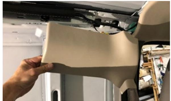
**B** Release the driver's side upper black wiring harness that is affixed along the whole length of the L/H inner roof rail body, you may need to pry some clips off to get this done
