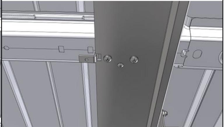
**G** Insert the feed the 1/4" x 1" bolts and spring washers through the anchor, through the OEM roof rail, and the thread on the brackets and tighten, this will secure or "sandwich" the anchor bracket to the roof beams resulting in a very strong anchor. Note, in some instances, you may need to carefully re-drill or elongate the OEM roof beam holes to match the ones on the roof anchor
